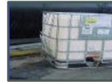
Damaged Cage and/or Pallet
